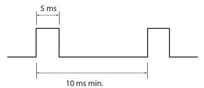
Note: The output cycle depends on the flow rate.
