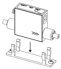
(3) Attach the upstream and downstream fluororesin tubes to the device as instructed below. Cut the tube  $\rightarrow$  Insert the union nut  $\rightarrow$  Insert the sleeve into the tube (a special tool is required)
