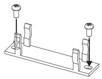
(2) Mount the main unit on the mounting bracket.
