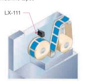
Detection of tapes stuck on copper foils
